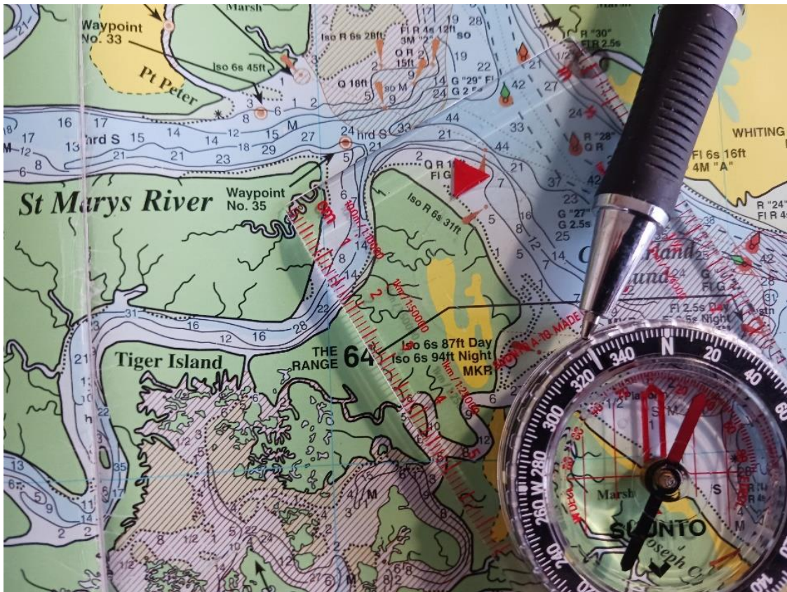
Figure 6. Read the number of degrees at the bearing line to find your course based on true north.
