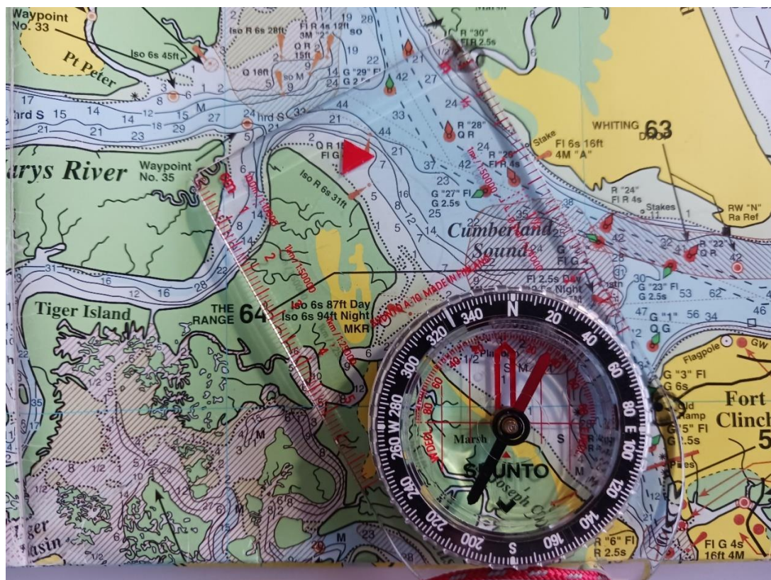
Figure 6. Turn the dial so that the several red orienting lines are parallel to the lines of longitude on the chart.
