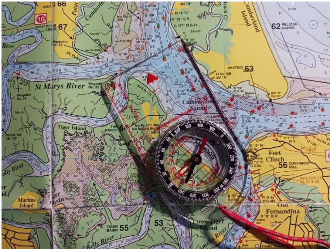
Figure 5. Connecting points A (put-in) and B (destination) with the edge of the compass
