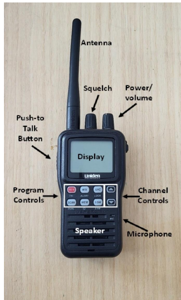
Figure 1. Components of a typical VHF radio
